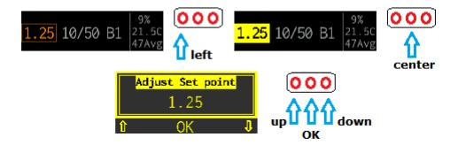
Adjusting the Set Point. Use up / down buttons, and press OK button to save.
