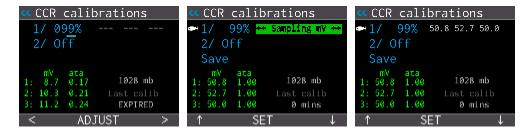
1 and 2 gas calibrate screens. Sample capture in progress. Set the high calibration mix percentage, start calibration, and saved sample.
