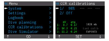
CCR calibrations. Line 1/ is the "high" O2 mix. Line 2/ is the "low" O2 mix used in calibrations.
